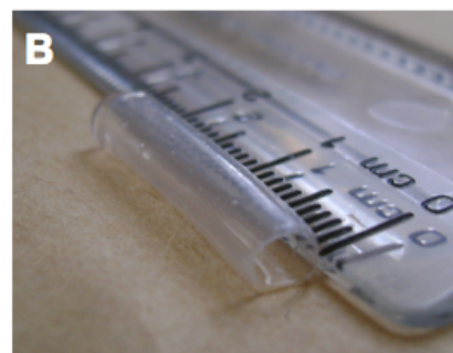
Figure 2: A) diagram of hollow microfiber with axial and cross-sectional views, B) hollow alginate stent after fabrication with a 1 mm brass rod.
