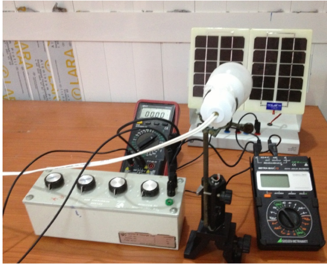
Figure 1: Experimental setup used for the photovoltaic investigation of non-shaded and shaded solar panels.
