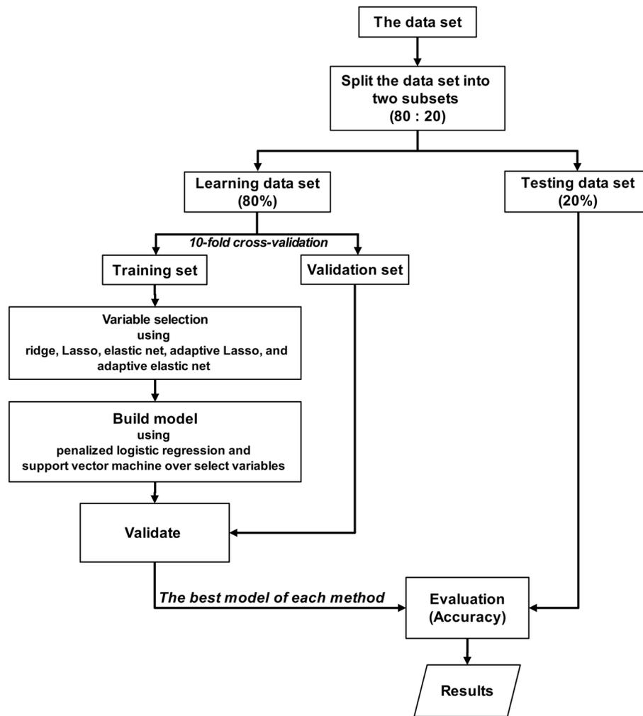
**Figure 2:** Workflow diagram of the machine-learning procedure.
